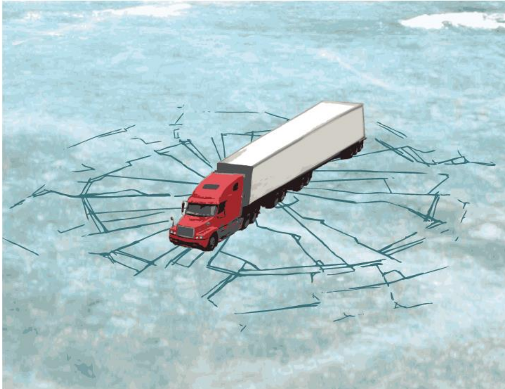
Figure 6: Aerial View of radial (spoke-like) and circumferential (round) cracks forming on overloaded ice
