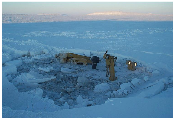
Figure 7 Breakthrough of a D10 Caterpillar tractor following formation of a circumferential crack pattern
